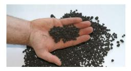
The USA dryer is capable of producing a Class A granular product by heating the biosolids, accomplishing a 90 percent total solids content. The temperature and total solids content values are in accordance with U.S. Environmental Protection Agency (EPA) Clean Water Act, Part 503 rule regarding land application of biosolids; those biosolids meeting the Class A requirement have less stringent regulations for reuse and disposal.
