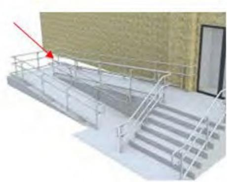
□ Handrails must extend a minimum of 12 inches beyond the ramp run or stairs. {DIB 82-06 4.3.10(8)}
