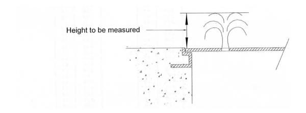
Example: Measured height of plume exiting pick/vent hole is 1 inch from a  $\frac{1}{2}$ -inch vent hole and there are 4 vent holes. The total volume per minute would be .94 gpm per hole (from attached chart) or 3.76 gpm total (.94 gpm x 4 holes) from the manhole cover. If the SSO lasted one hour, the total wastewater lost would be 226 gallons (3.76 x 60 = 225.6).
