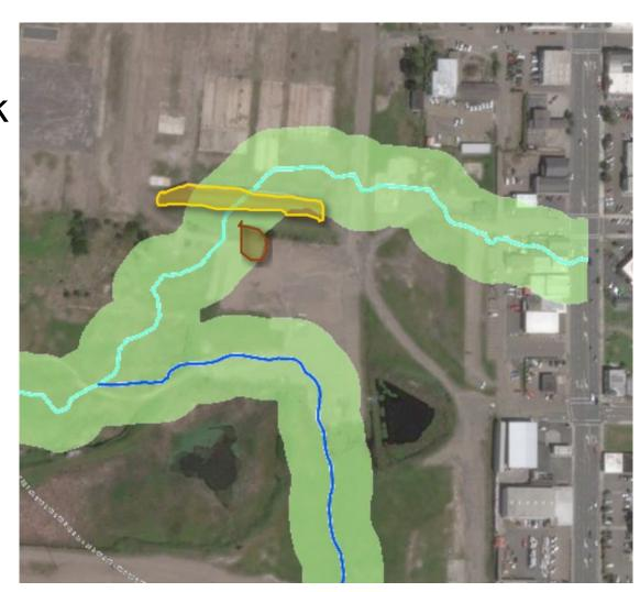
Figure 2B: Straight line route of a daylighted Alder Creek, might be too steep to handle the Head, and the "Fire Station Meander" route based on topography, along with excavation of the Eastern edge of the Ramp:
