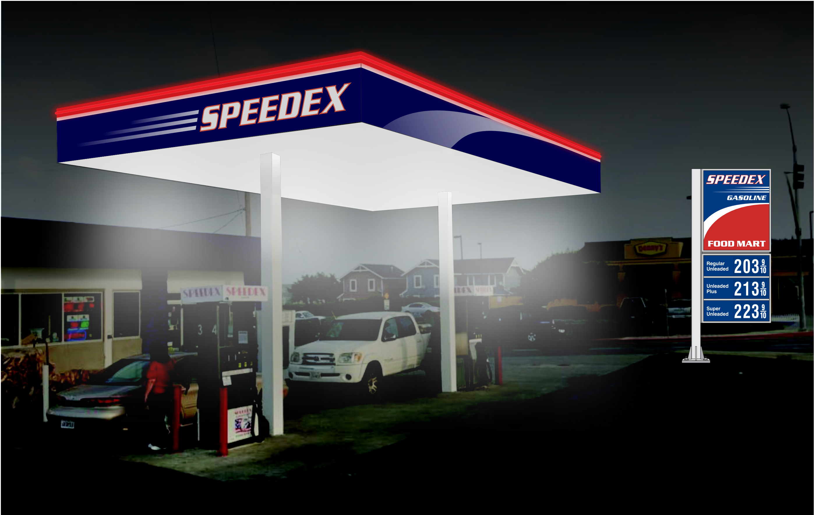
NIGHT RENDERING OF PROPOSED NEW VINYL GRAPHICS, LED BORDER TUBE ILLUMINATION & NEW DOUBLE-FACE ILLUMINATED SIGN w/ ZIP-TRACK FUEL PRICE DISPLAY
