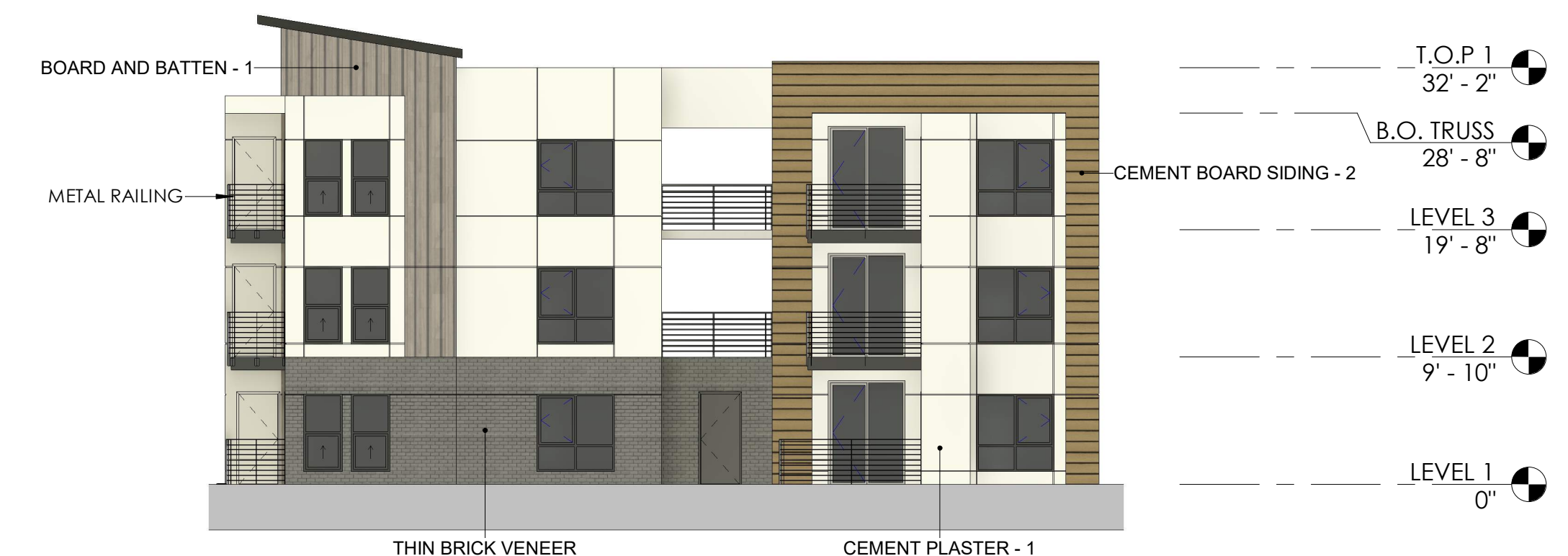
BLDG 1 - SOUTH ELEVATION
