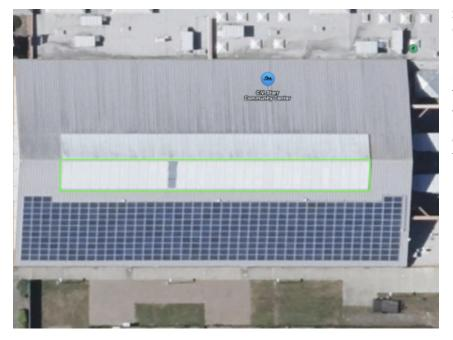
Southern facing side of CV Starr Community Center Kingspan Skylights have been found to be faulty and in need of replacement. Some Panels have failed seals and were never replaced or maintained over the prior 15 years that the skylights were in place. Some skylights are still in working condition but are also be replaced for equal quality of materials. Those extra panels are to be removed and kept for future use if necessary. \*Prevailing Wage Work.
