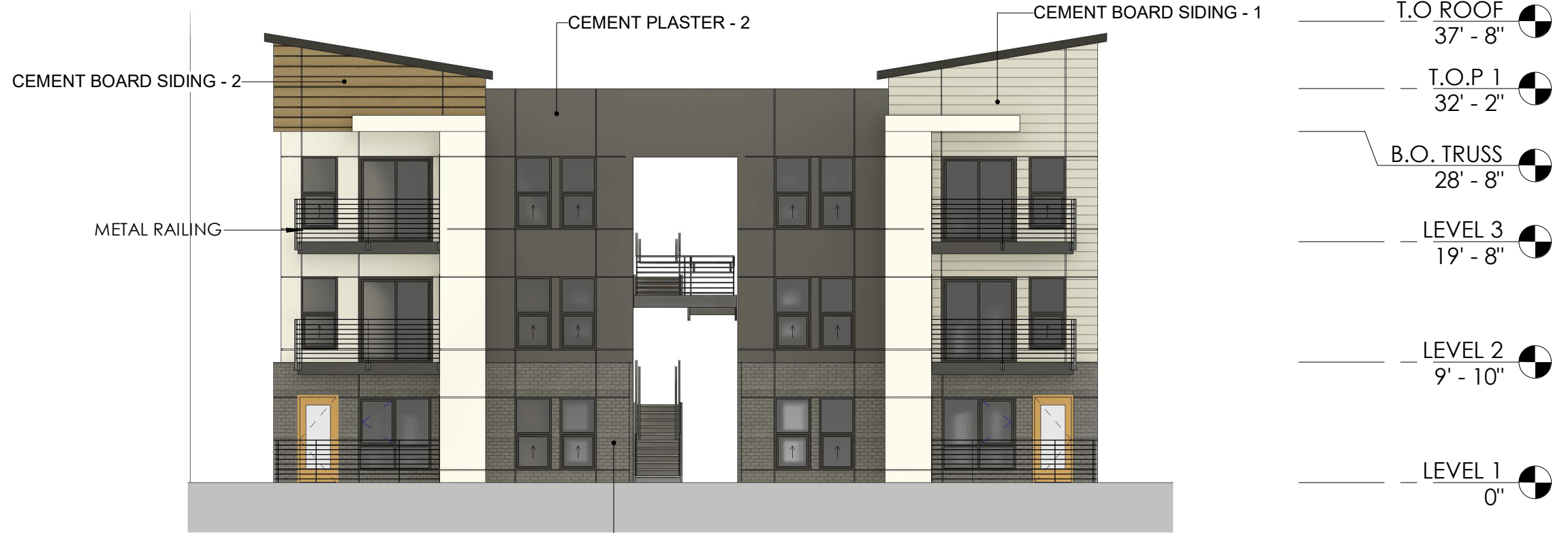
BLDG 5 - NORTH ELEVATION
