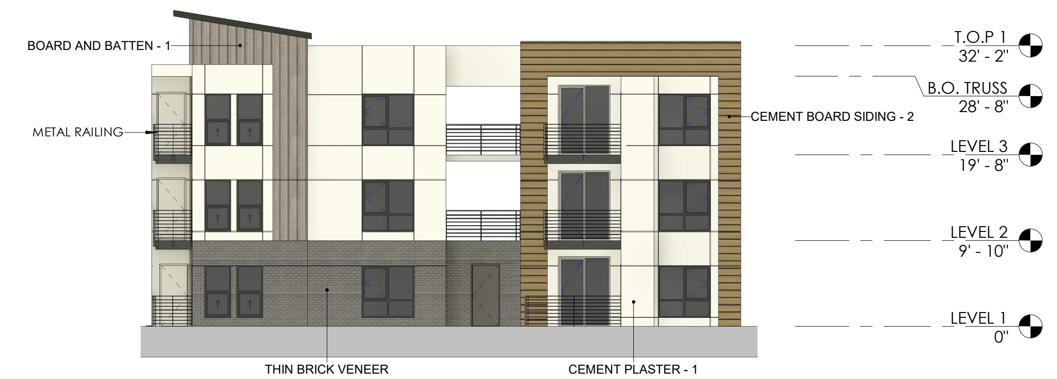
BLDG 1 - SOUTH ELEVATION
