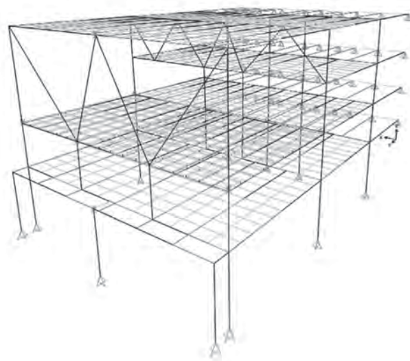
(b) Floor with transfer trusses
