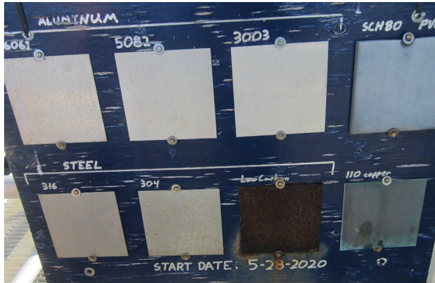
Figure 7-1. Corrosion Potential Coupon Testing at the WWTF.
