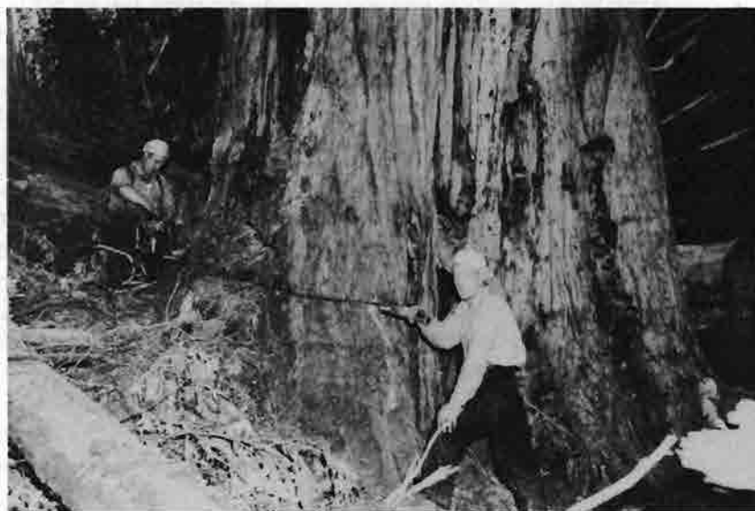
Though still called "choppers," today's tree-fallers use power-driven chain saws instead of axes and the old "cross-cuts."
