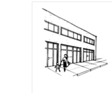
Without architectural variations buildings appear flat, larger, and "box like"
