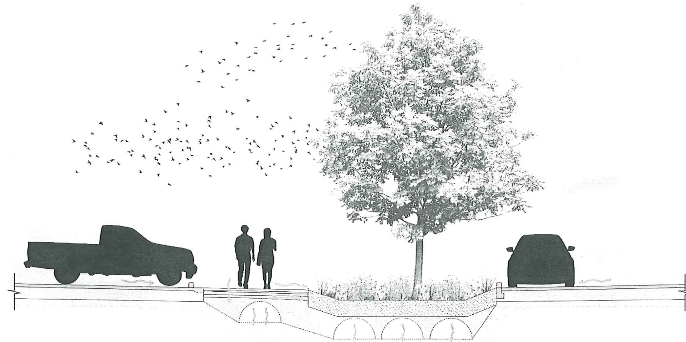
ILLUSTRATIVE CROSS SECTION OF BIOFILTRATION SYSTEM AND PARKING LOT NOT TO SCALE
