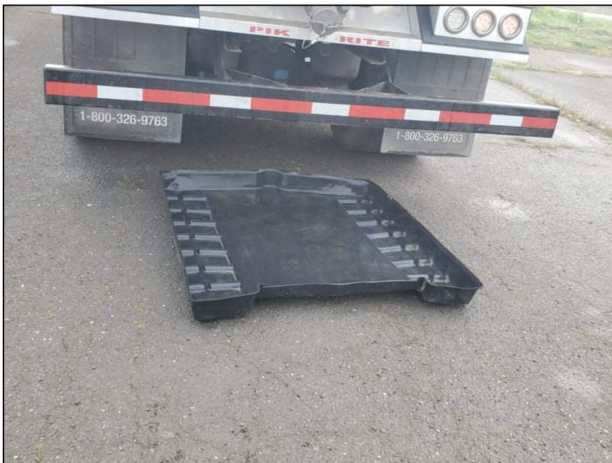
Containment tray for truck to truck waste transfers
